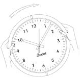
Once the the bracket (wall or double-sided) is installed, turn the clock a quarter turn in the clockwise direction so that the clock is in the correct position.
