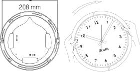
Once the the bracket (wall or double-sided) is installed, turn the clock a quarter turn in the clockwise direction so that the clock is in the correct position.
